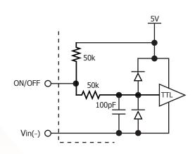
Figure B: Internal ON/OFF pin circuitry
