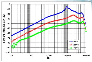
**Figure 14:** Magnitude of incremental forward transmission (FT =  $v_{out'}$ ) for minimum, nominal, and maximum input voltage at full rated power.
