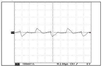
**Figure 10:** Output voltage ripple, Vout, at nominal input voltage and rated load current (100 mV/div). Load Capacitance: 1 μF ceramic capacitor. Bandwidth: 20 MHz. See Figure 17.
