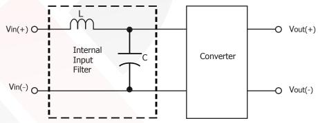
Figure E: Internal Input Filter Diagram
