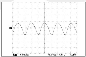
Figure 9: Input terminal current ripple, i<sub>C</sub>, at full rated output current and nominal input voltage with SynQor MCOTS filter module (1 A/div). Bandwidth: 20MHz. See Figure 17.
