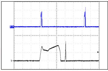
**Figure 18:** Load current (50A/div) as a function of time (2ms/div and 40ms/div) when the converter attempts to turn on into a 10 m $\Omega$  short circuit.
