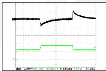
Figure 11: Output voltage response to step-change in load current (50%-75%-50% of lout(max); dI/dt = 0.1 A/µs). Load cap: 1 µF ceramic capacitor. Ch 1: Vout (200mV/div), Ch 2: Iout (20A/div).
