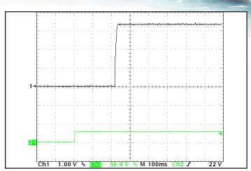
Figure 8: Turn-on transient at full resistive load and zero output capacitance initiated by Vin. ON/OFF Pin previously low. Ch 1: Vout (1V/div). Ch 2: Vin (50V/div).
