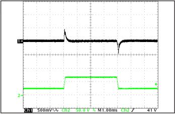
**Figure 12:** Output voltage response to step-change in input voltage (500V/ms) at full load current. Load cap: 100 μF electrolytic capacitance. Ch1: Vout (500mV/div), Ch 2: Vin (50V/div).
